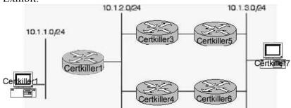
Routers Certkiller 5 and Certkiller 6 are configured for HSRP (Hot Standby Routing Protocol). Certkiller 5 has a priority of 100, while Certkiller 6 has a priority of 50. At one point, when Certkiller 5 is the active router, it fails, and Certkiller 6 takes over as the active router. A few minutes later, Certkiller 5 returns to service. What happens?
