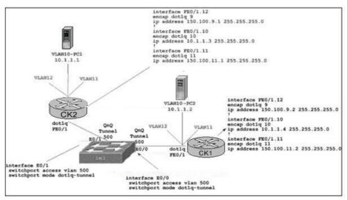
The exhibit shows the SW1 topology and configuration. When the show vlan command is executed on SW1:
