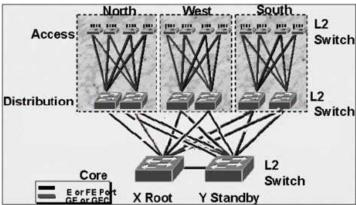
The diagram shows an L2 switched campus. Switch X is the STP root and switch Y is the standby root. How many of the links in the diagram will be placed in blocking mode by STP?
