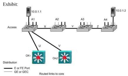
The diagram shows a wiring closet stack of four L2 switches A1, A2, A3, and A4. A1, A2, A3 and A4 are connected in series. Switch A1 is the root switch and connects to CK1 and CK2. There are no loops in the wiring closet VLAN (=subnet). The architect wants to remove X, Y and Z, and connect A1 directly to A2, A3, and A4 in s star. Is this a good idea?
