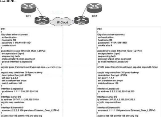
Observing the shown configuration, assume PE1 and PE2 already have IP connectivity, what behavior should be expected?
