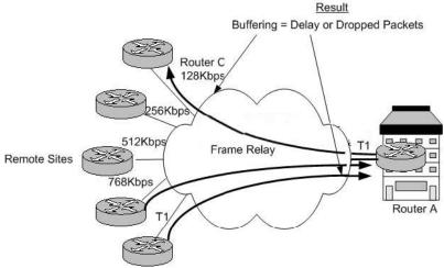
In the diagram shown, what mechanism needs to be employed on the remote site routers to aid congestion avoidance in the core, based on traffic properties?
